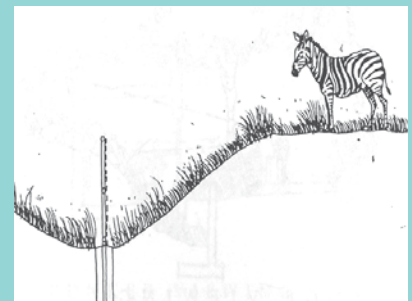
Depressed vertical fence barrier
